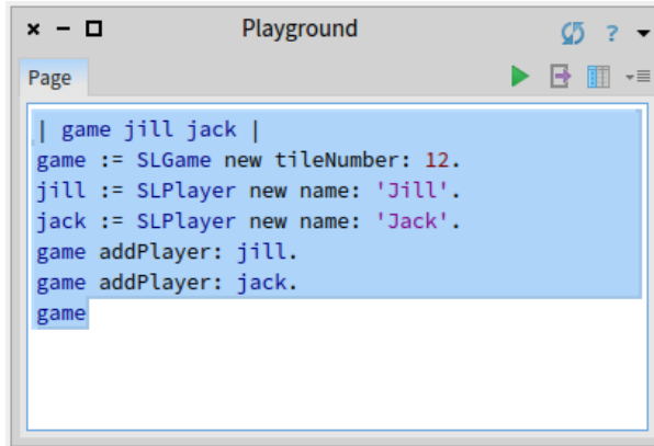
Figure 18-2 Playground in action. Use Do it and go - to get an embedded inspector.
